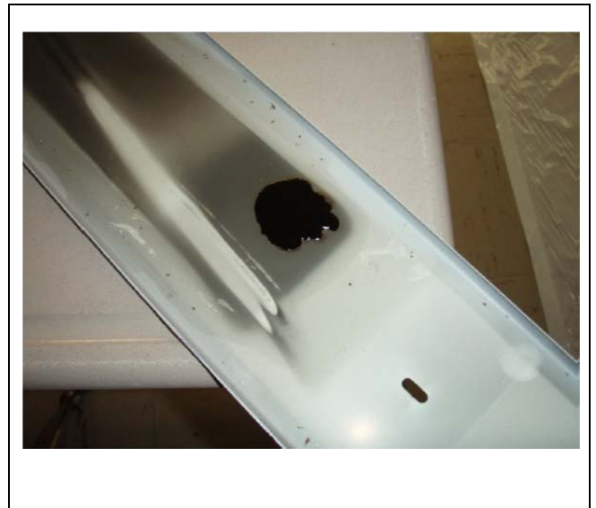
Figure 2-2d: Leaked Potting Material from FLB (USEPA, 2013b)
