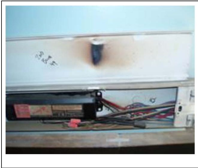
Figure 2-2a: Example of a Burst FLB (USEPA, 2013b)
