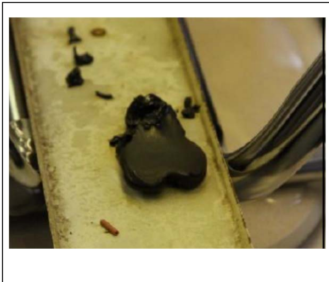
Figure 2-2c: Tar-like Potting Material from Failed FLB (USEPA, 2013b)
