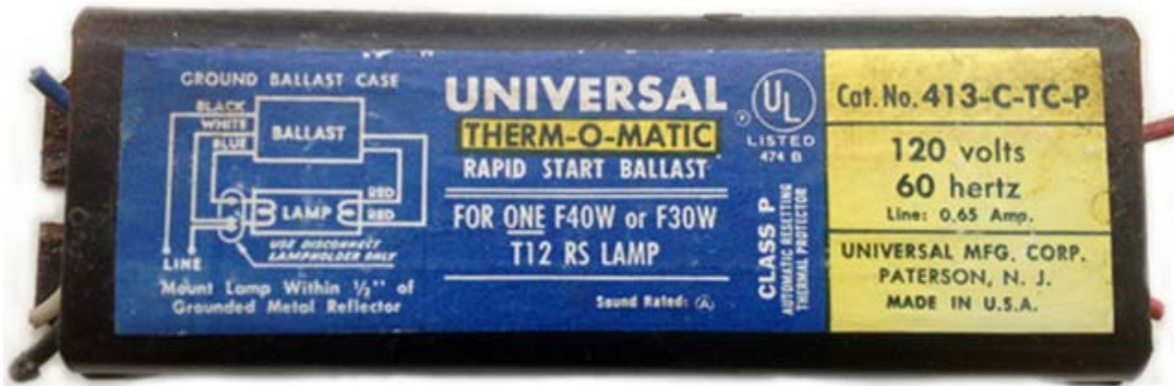
A typical pre-1979 PCB-containing fluorescent light ballast (FLB)
